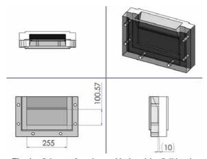
Fig. 1. Schema of casting mold plotted by Solidworks software. (unit:mm)
