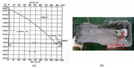
Fig. 5. (a) Si-Al phase diagram; (b) The macro-segregation of Si-Al ingot.
