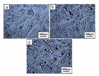
**Fig. 4.** The OM image of Si-Al targets containing different Al contents: (a) 25wt.%; (b) 30wt.%; (c) 35wt.%
