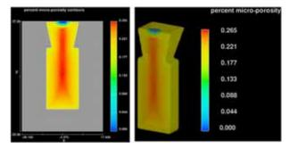
**Fig. 6.** Results of Flow-3D simulation of Si-Al alloy cast into a thick mold.
