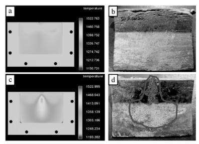
Fig. 9. Relation between the temperature distribution of melt and shrinkage pores on the surface of an ingot.
