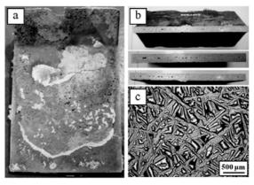
**Fig. 11.** Shrinkage pores on the (a) surface; and (b) center of Si-30wt.%Al ingot cast with the condition of 1330 casting temperature and 300 mold temperature. (c) OM observation and the distribution of shrinkage pores.
