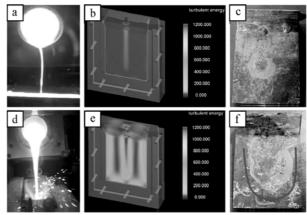
**Fig. 16.** Relation between the pouring flow of melt and the casting defect on the surface of the ingot.
